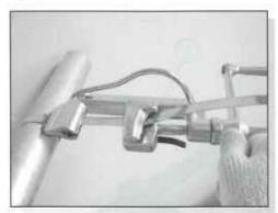
When desired tension is reached, swing tool over buckle. This movement increase tension of band and, to avoid breakage, handle must be reversed slightly as tool is swing over.
