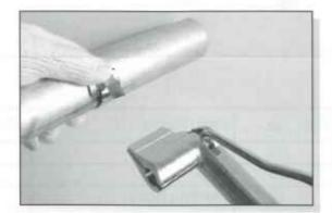
Remove tool, whilest holding band down with thumb.
